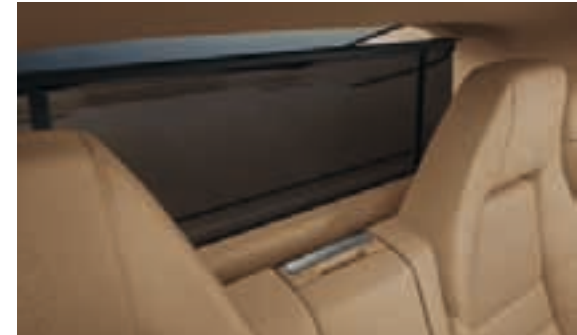
Removable luggage compartment cover with electric roll-up sunblind for behind the rear compartment
