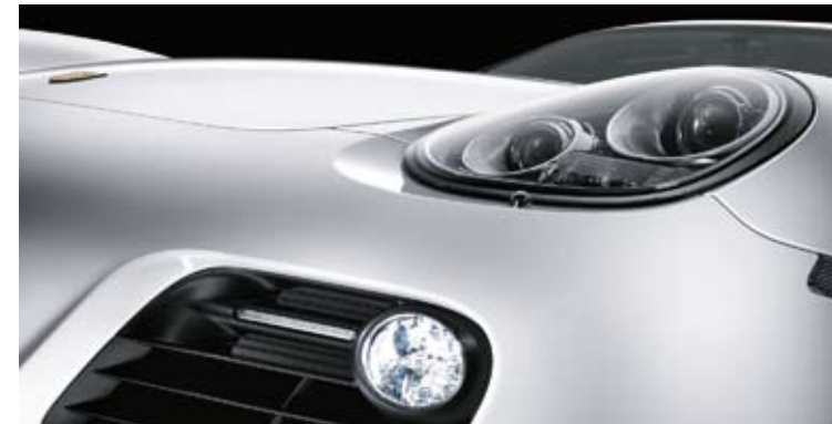
Bi-Xenon headlights with dynamic cornering lights and LED daytime running lights
