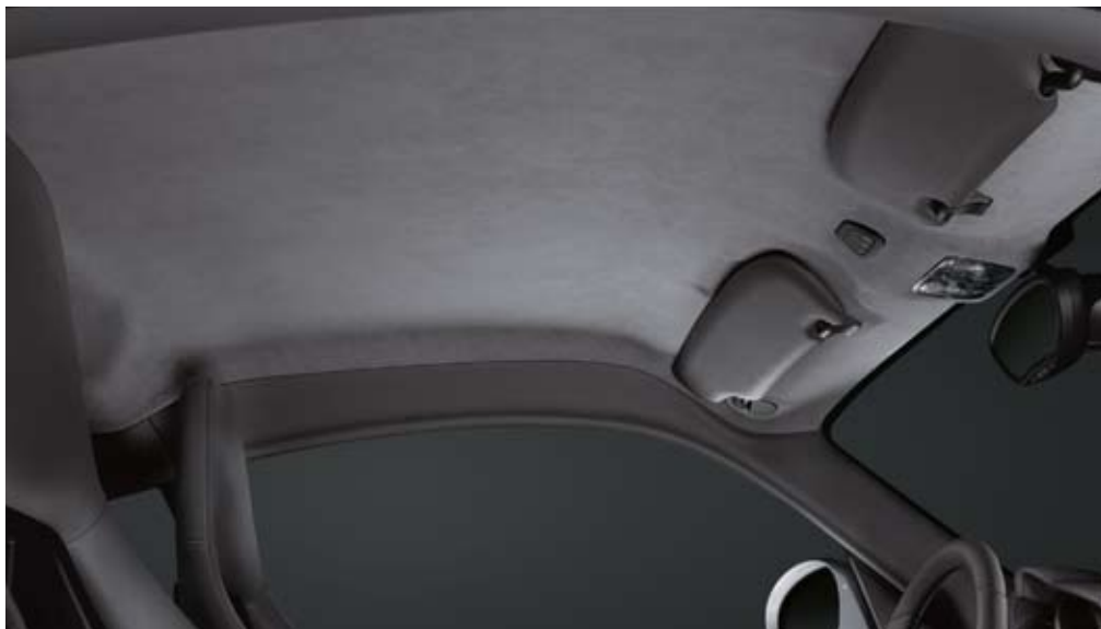
Rooflining in Alcantara
