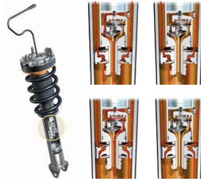
Left: Rebound in 'Normal' mode – working piston and bypass, sporty-comfortable tuning Right: Rebound in 'Sport' mode – working piston only, sporty-hard tuning
