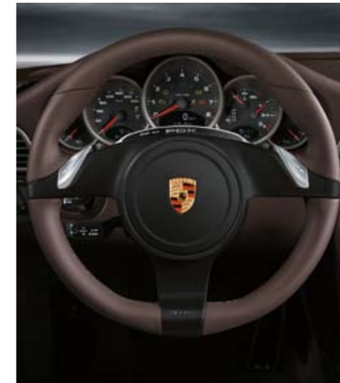
Three-spoke sports steering wheel with gearshift switches in combination with PDK and Sport Chrono Package Plus
